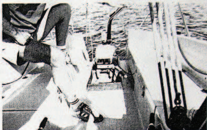
LEFT: Mainsheet traveller tack is recessed in bridge deck.
