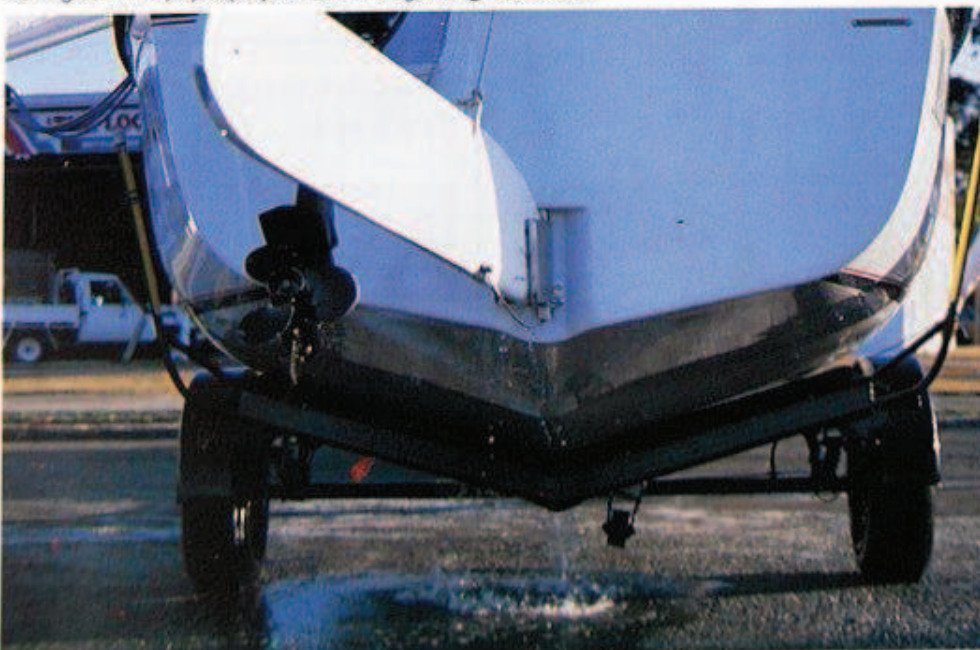
On the trailer, ballast water draining away.
